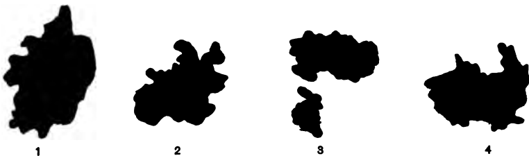
CONTACTS OF 36-IN. STEEL-TIRED WHEEL UNDER CAFÉ CAR. WEIGHT ON WHEEL, 6,075 LBS.
